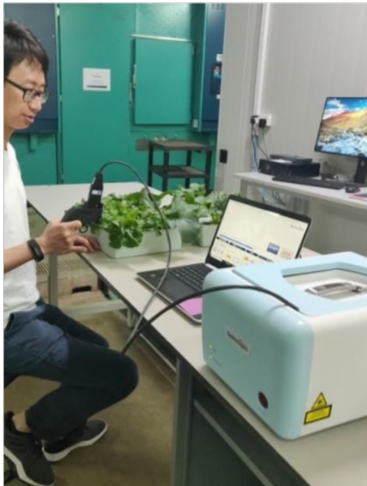
Portable leaf-clip Raman sensor being used at TLL to detect nutrient stress in leafy vegetables. Photo Credit: Singapore-MIT Alliance for Research and Technology (SMART)
